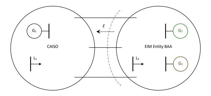
The power transfer (*E*) between the BAAs is limited to 100MW. The resource data is as follows:
